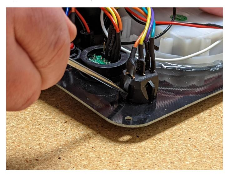
10. Remove the connector with the yellow and orange wires from the power adapter. Lightly press in the tabs securing the blue and orange wires and remove the wires from the connector. Completely remove the power switch and all wires from the old faceplate at this point.
