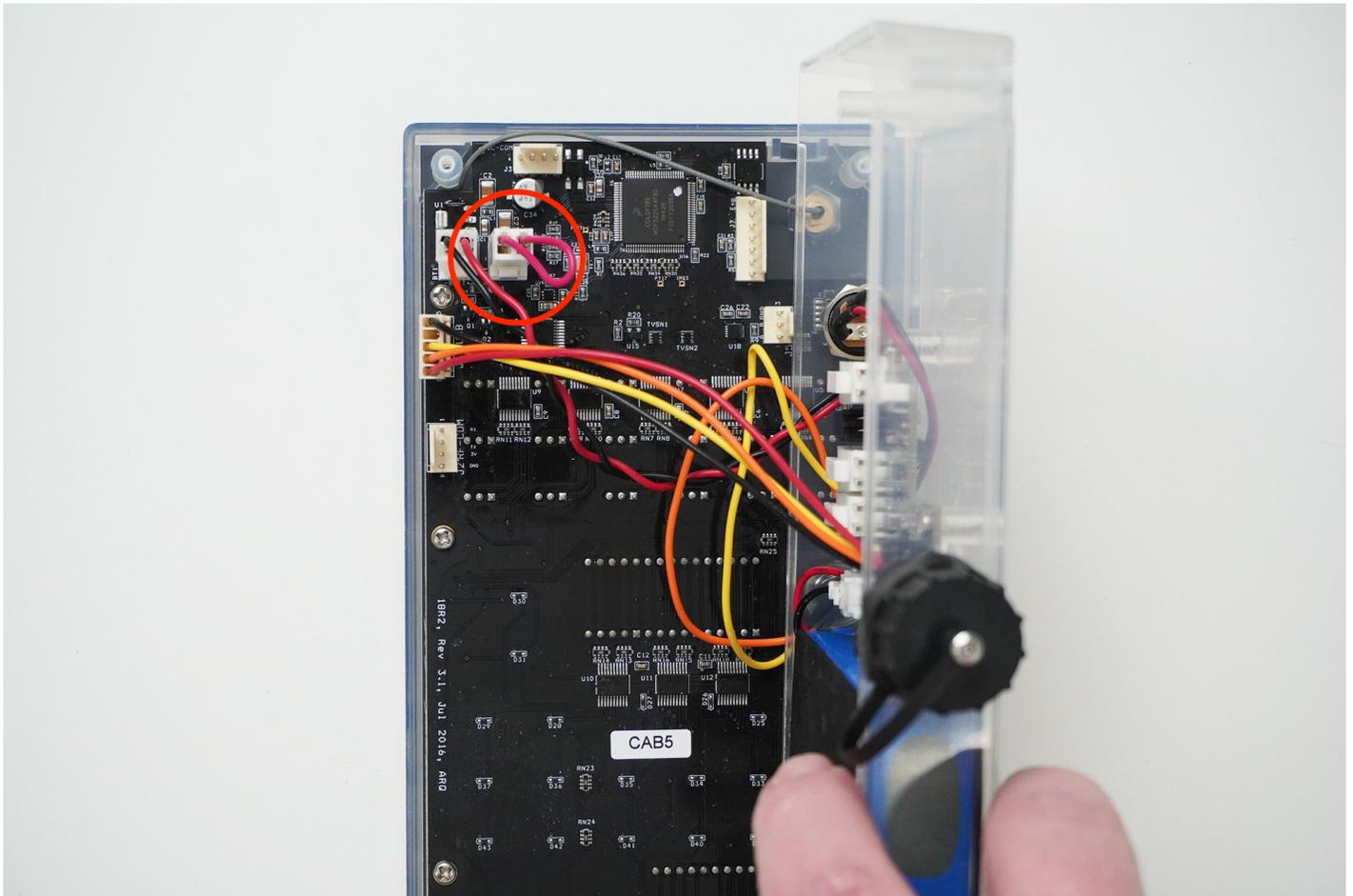
**11.** Make sure no wires are being pinched and place the back enclosure back on the 18R2. Reinstall the four back enclosure screws.
